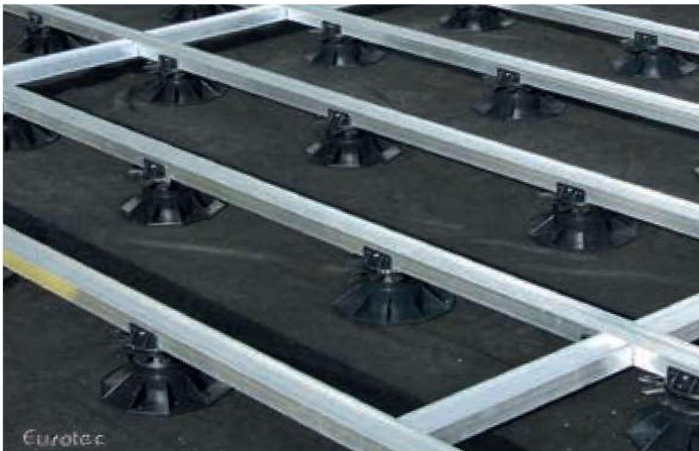
The Aluminum System Profile tracks are 13'-1-1/2" (4 meters) long. Connectors are provided for longer runs as needed. Always place a pedestal directly beneath each connection for proper support.
